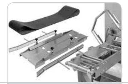
Sanitary design in-feed can be easily disassembled without tools.
