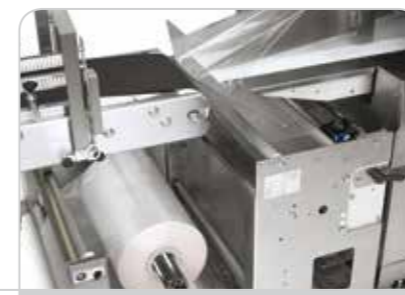
Front loading reel holder with pneumatic fastening.
